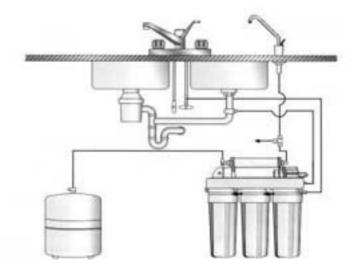
This system may be mounted in either a vertical or horizontal position and must be positioned to allow access for service and filter cartridge changing. At the same time, the assembly should be relatively near the spigot to maximize flow rate.
